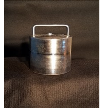
Figure 9: ASTM F355 A Missile
