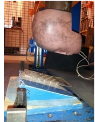
Figure 7: 50th Percentile Male Hybrid III FHM
