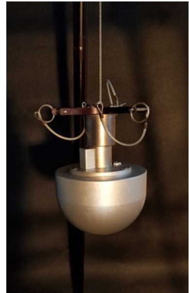
Figure 4: ASTM F355 E Missile
