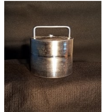
Figure 8: ASTM F355 A Missile
